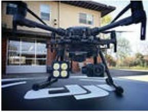
DJI drone with a thermal-imaging camera designed by FLIR Systems
